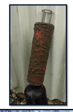
OWMS failure103"Failures"/yr13Total no. of OWMS37,000% failure/yr0.035%~800/yr
