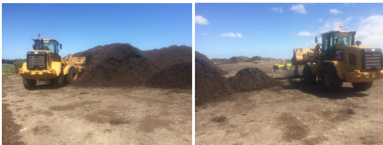
Figure 4.1.1 A Front-end loader is used to remove the four corners of each compost pile to allow for representative samples to be taken.
