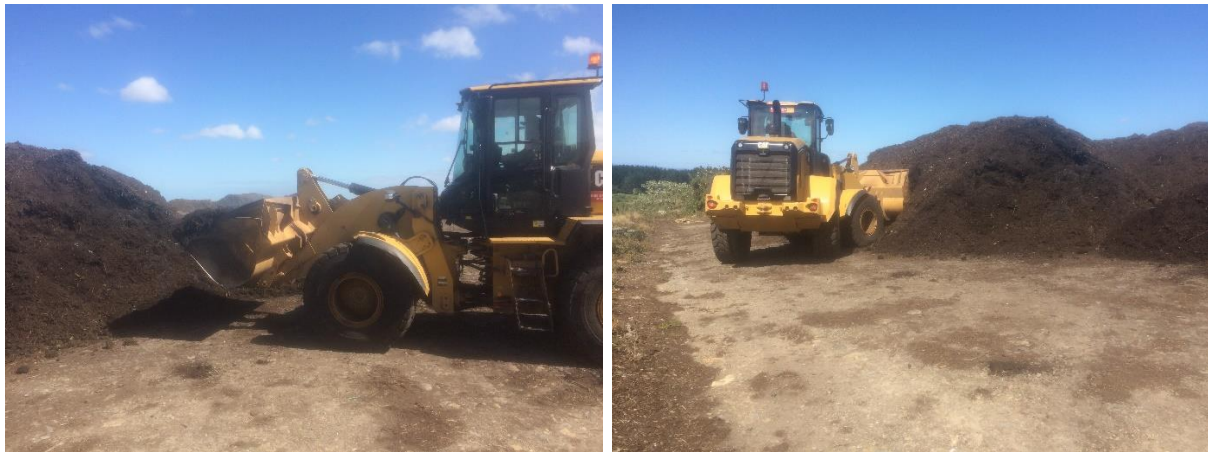
Figure 3.4.1. A front-end loader mixing green waste for windrow 6 (WWTP digested sludge with green waste) in February 2019.
