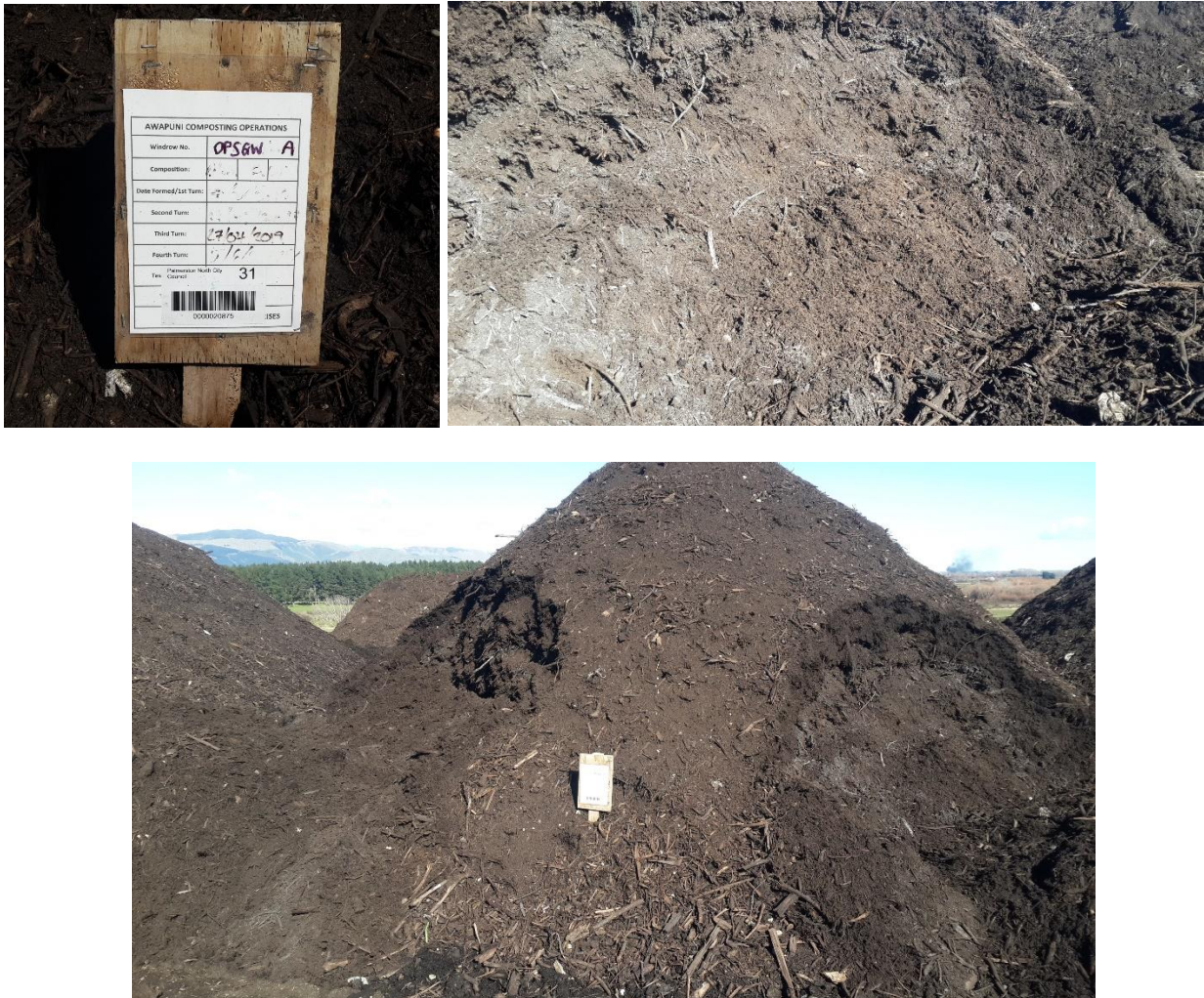
Figure 4.8. Windrow 3, PNCC alum sludge + green waste. Photos taken on 5 th August after 4 months of composting.
