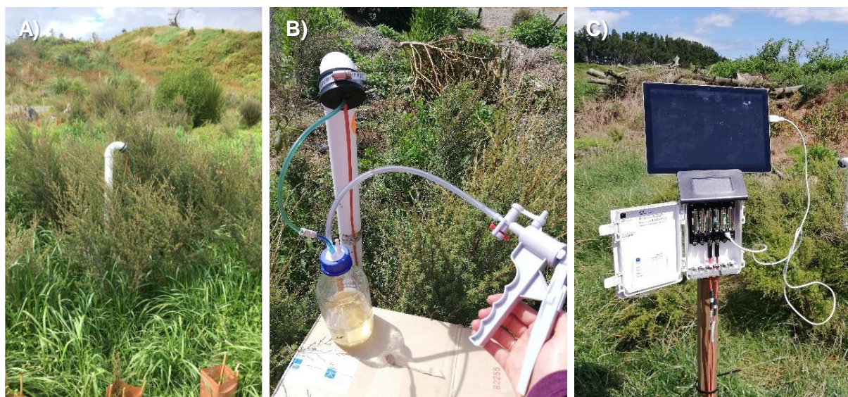
Figure 9 A) WFM with kānuka plants; B) Collecting leachate samples from the WFMs by handpump; C) Retrieving data from the data logger.
