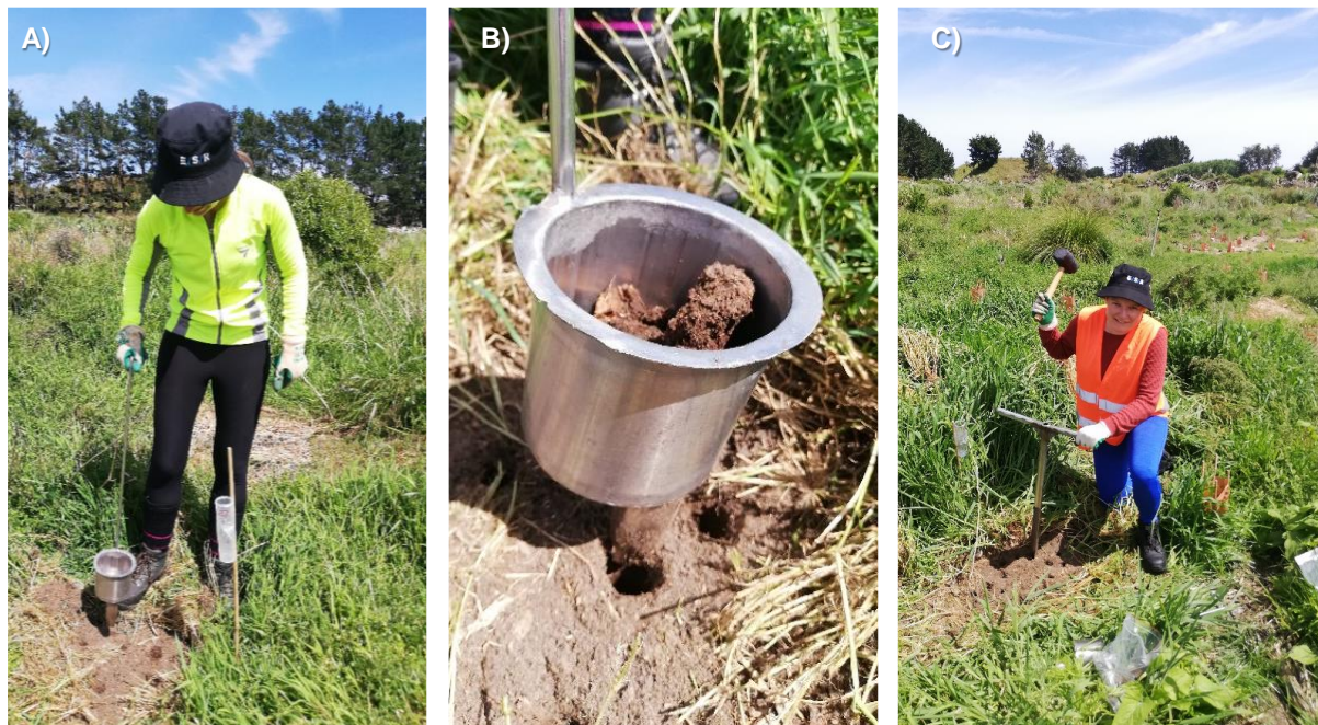
Figure 7 A) Collection of soil sample from the top soil (0-10 cm) with a bucket soil sampler; B) pooled sample in the bucket soil sampler; C) Collection of soil sample from the sub soil (30-45 cm) with a soil corer
