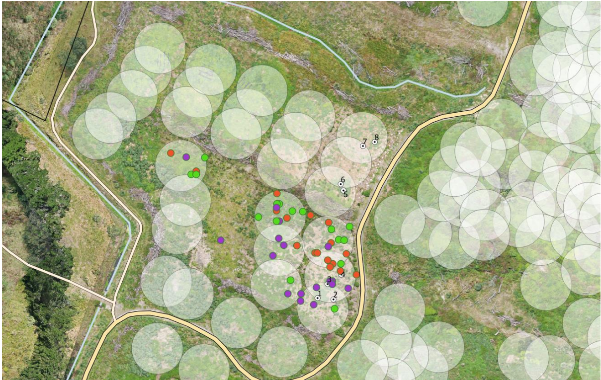
Figure 5 Aerial image showing the reach of the irrigation sprinklers in white circles, and sampling points in small red circles (mānuka), green circles (kānuka) and purple circles (pasture). Numbered points show the location of the Water Flux Meters (WFMs, Section 3.5).
