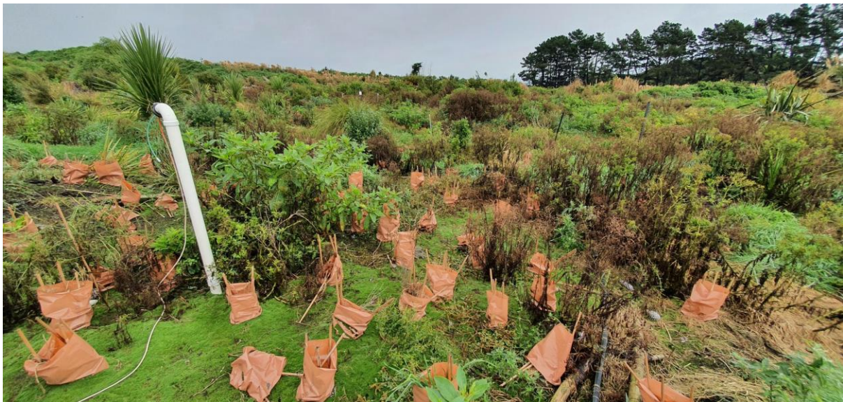
Figure 27: All kānuka and other higher plants on two of the lysimeters had died, leaving a cover of moss.
